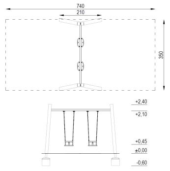
**COMPONENTS: MATERIALS:** Supporting structure 1 set Construction poles: recycled material Basket seat 2 pcs Steel elements: galvanized steel, powder coated Basket seat: made of steel construction, coated with rubber Chain: stainless steel, calibrated Caps: plastic Foundations: concrete min. C12/15 standard
